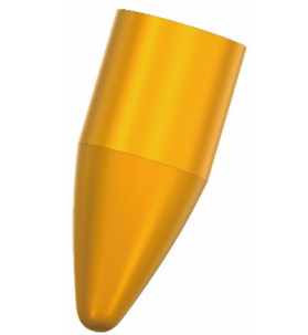
图7 新设计指状铣刀 Fig. 7 Newly designed finger milling cutter
